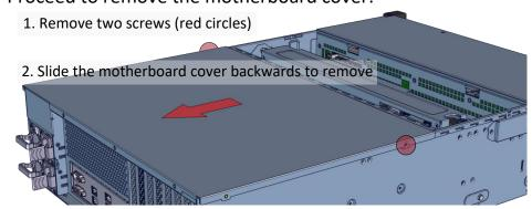
**4. Inspect the Inside** of the unit. Internal components comprise of a Tyan motherboard, an expander board, optional rear 2x and 4x 2.5" bays, 4x internal fan modules (electronically attached to the motherboard).
