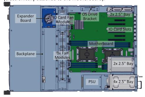
To install OS disk(s), a space for 2 OS disks is available on the left inner wall of the chassis.
