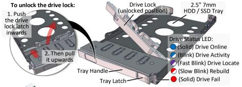
Tool-less drive tray is best used for SSDs. It is recommended to apply M3 screws when installing HDDs
