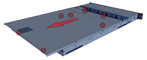
**4. Inspect the internal** of the chassis. By default, it consists of:
