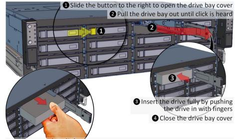
To remove the disk, open the drive bay cover, pull the handle out so that disk slightly slide out, and pull out the disk with hand.
