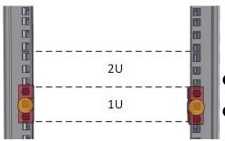
Red rectangles are locations for slide rail position (front and rear posts) Place square nut at yellow circles for enclosure screws (front only)
