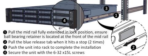
For a complete instruction on how to install unit to the rack, please follow the Slide Rail Installation Guide.
