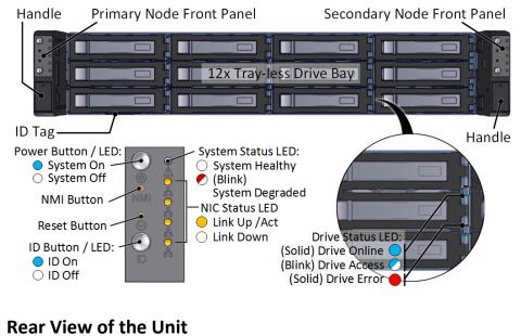
**3.** Install 2.5" Drives to the unit as illustrated. It is suggested to install HDDs after the unit is mounted to the rack.
