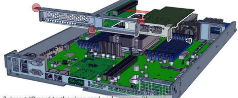
2. Insert IO card to the riser card and secure with screw 3. Place riser card assembly back to enclosure
